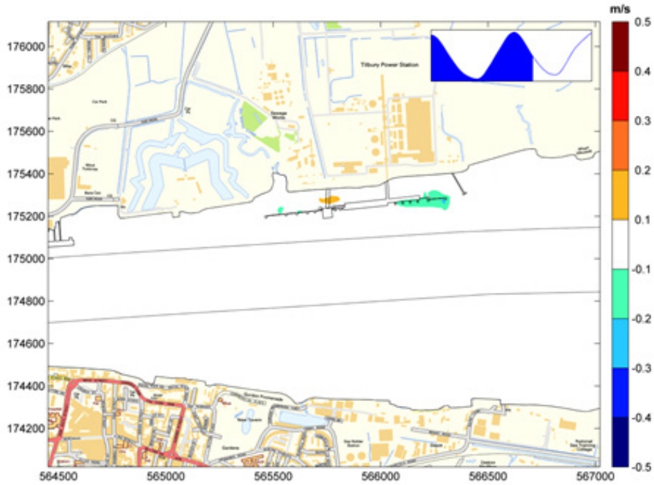
Figure 2.22 Difference in current speed magnitude - proposed works compared to baseline, near surface, peak ebb tide
