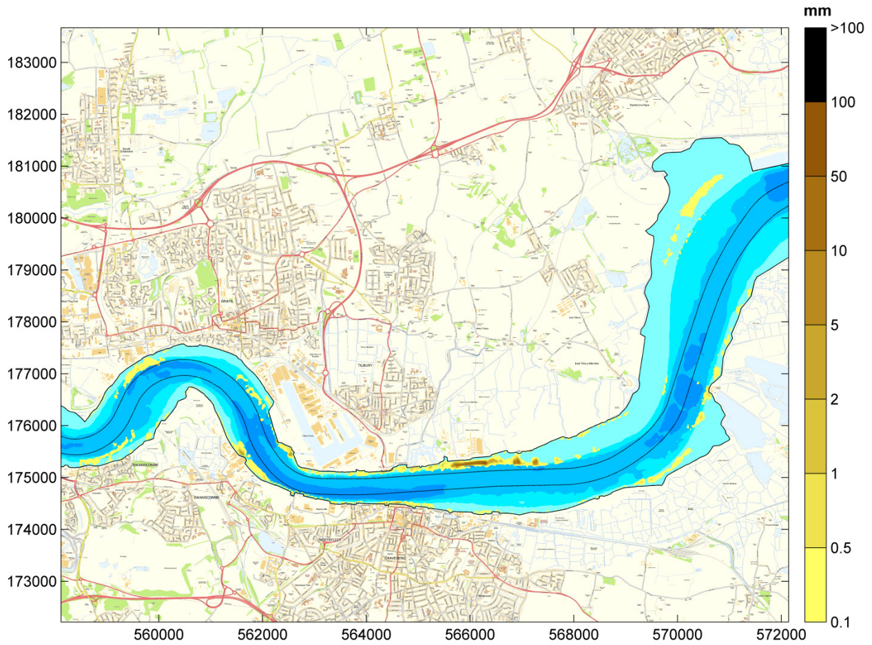
Figure 4.8: Maximum deposition depth of the released sediment during 14 days of backhoe dredging Background image contains OS data © Crown copyright (2016)
