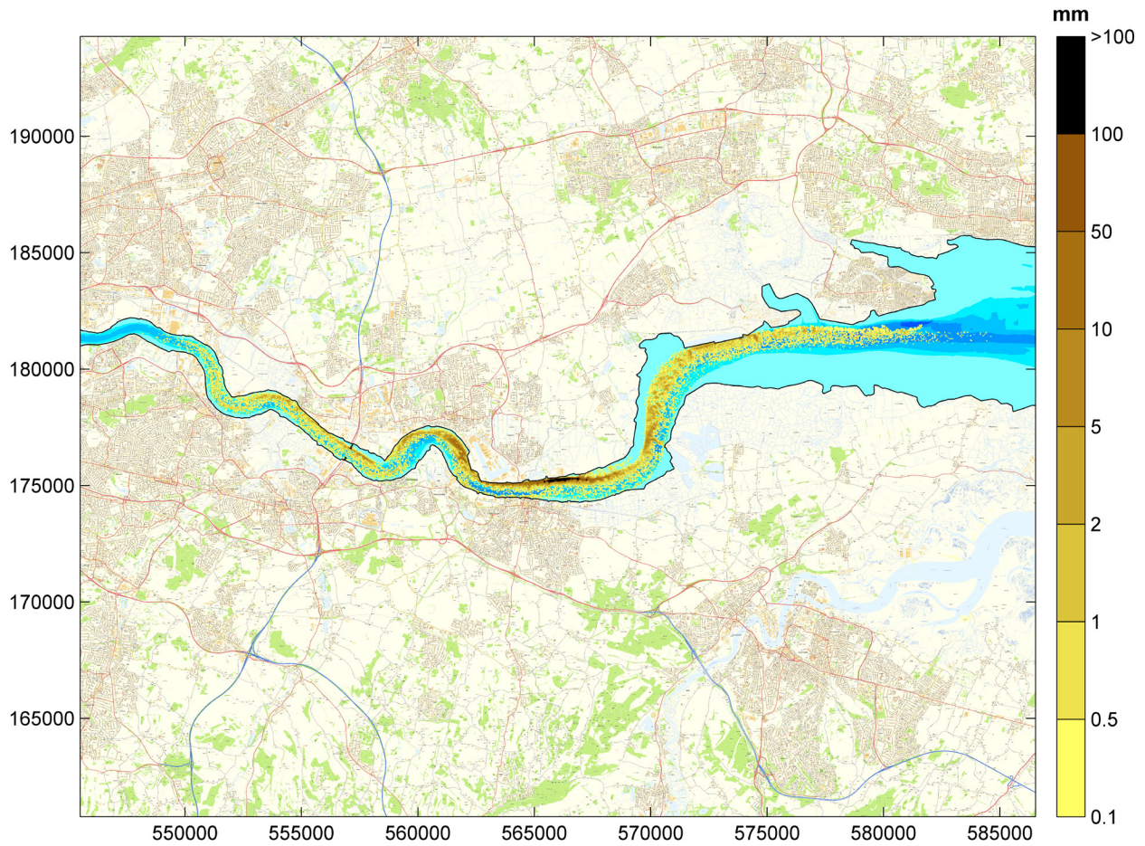
Figure 4.17: Nett accumulation of the released sediment at the end of 14 days of WID – Scenario 1
